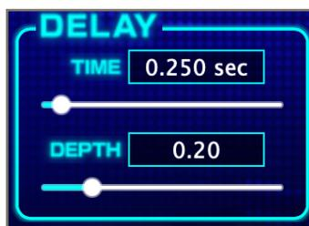
Creates an echoing effect by delaying the sound. The JACPOTSYNTH8 has internal settings optimized to make sounds in the center of the PAN field sound clear and pristine. Try using it with reverb on lead instruments for main melodies or sound effects. You'll be amazed at how beautifully it resonates.
