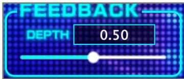
Routes the output signal back into the input, creating self-oscillation and resonant effects. This is a unique routing feature of the JACPOTSYNTH8. Try combining it with the FILTER, DISTORTION, and other effects.
