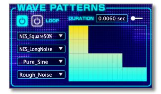
Sequentially switch between up to 4 different OSC waveforms. The interval between switches can be set using the dedicated dots and slider.
